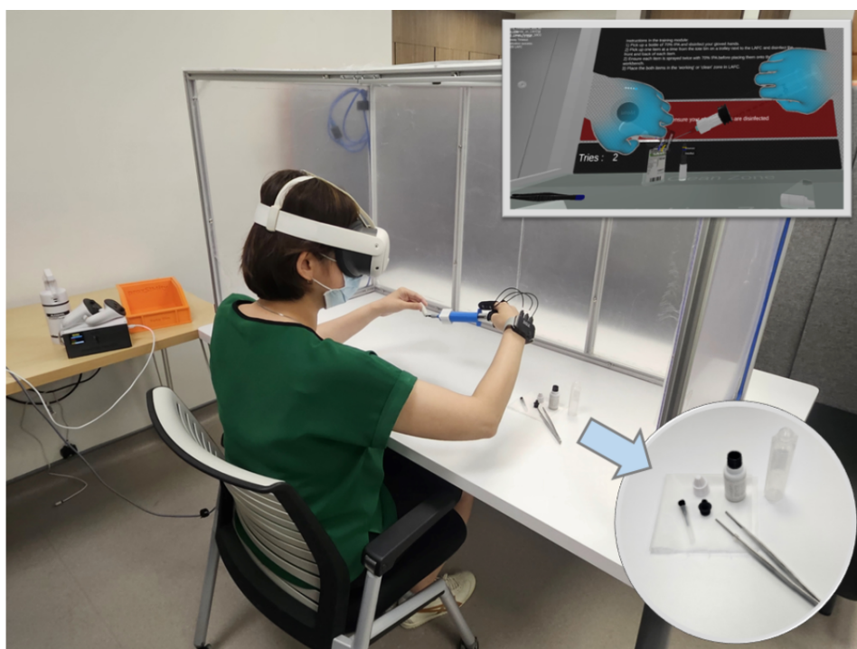
Fig 1. VAC set-up with 3D-printed items, showing the process of drawing liquid from a syringe. (Person in picture: Ms Jacelyn Han)
