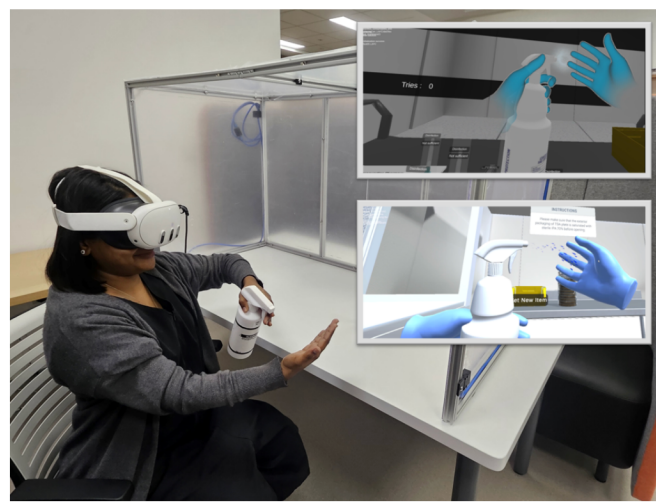
Fig 3. VAC set-up showing the process of disinfecting gloved hands. (Person in picture: Ms Shakunthala D/O Hans Raj)
